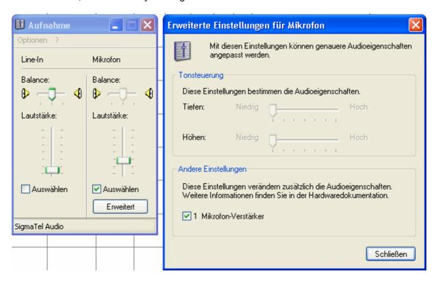
In the next step the Win-mixer is called up. In the RECORD menu the microphone is chosen. With the button EXPAND the menu is EXPANDED and OPTIONS for microphones is opened. Here you click on microphone amplifier. The options are also called Mic-boost or +20dB.
