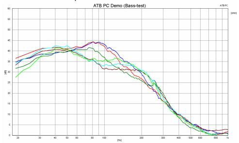
The measurements show the frequency sweeps of the subwoofer. The red and blue curves show a too strong over-rise. The green curve is ideal. The light green, light blue and brown show a deletion.
