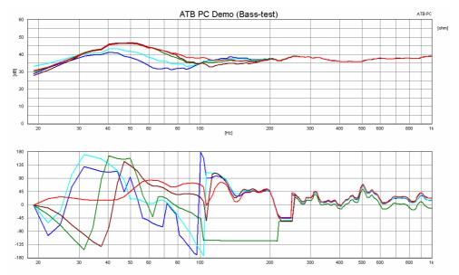
In the phase frequency sweep the different acoustical phase sweeps of the main speakers and the subwoofer are illustrated. The blue curve shows the  $180^{\circ}$  turn of phase. The phase setting of  $0^{\circ}$  is shown with the red curve. At  $0^{\circ}$  the frequency sweep is the best balanced. The  $0^{\circ}$  setting is only for this single loudspeaker the right one.
