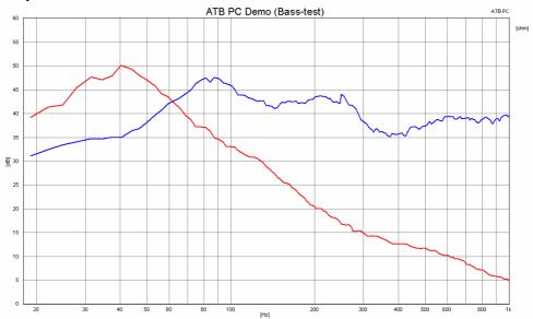
The red curve shows the subwoofer and the blue the main speaker. On the subwoofer crossover, the crossover frequency and sound level are setup, so that both curves accomplish each other. The sound level frequency curves of the speakers fit well together. When the loudspeakers are run together, the phase frequency curves also have to fit each other.
