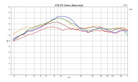
The picture shows the first measurement. The positioning of the loudspeakers in the room is measured. On the first measurement, the speaker stands in the corner of the room, blue curve. On the next measurement, the speaker is turned to one side. The second
