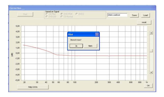
After saving, the correction curve is available for all following measurements and is automatically loaded at the start of the program.
