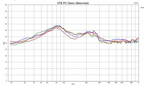
In the picture the frequency response of the main loudspeakers with different distances to the sidewalls are illustrated. The brown curve shows the corner position. With the blue curve, the distance measures 18cm, with 36cm distance green and 54cm red the difference is minimal.
