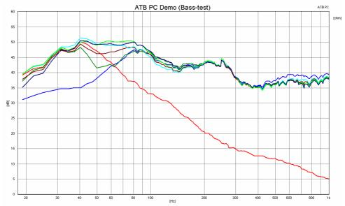
The picture shows the resulting frequency sweep with different phase settings of the subwoofer crossover. The green curve with a 180° setting of the controller creates a large breakdown. The brown curve with 90° looks a lot better. The next settings up until 0° can not exactly be judged. By ear though, there is still a big difference between the settings. This is due to the impulse response that is only correct when the phase curves fit.
