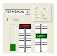
With the linear level controller (Record), you can set the sensitivity of the microphone. The green bar should fill the display to one quarter.
