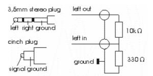
After connecting the test adapter, for internal system correction the BMH signal with a frequency range of von 20Hz to 20kHz is switched on.
